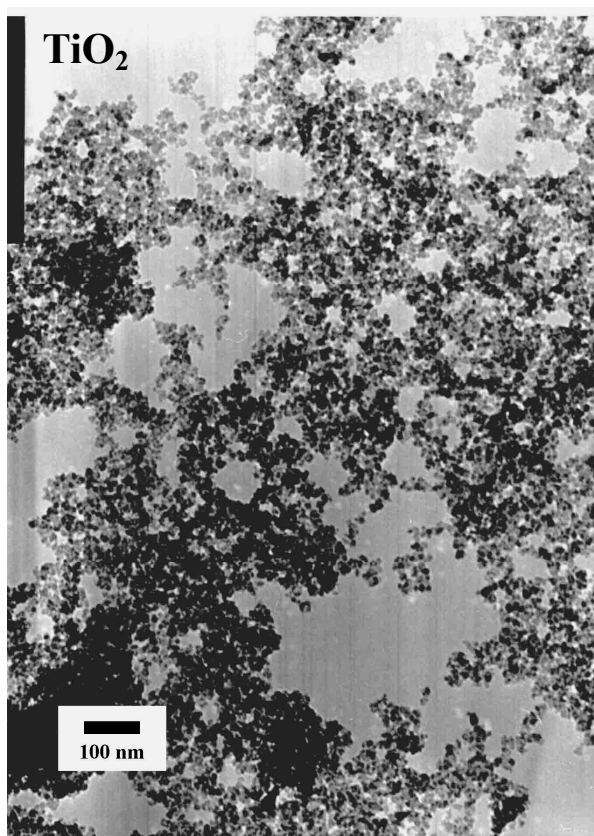
Figure S2 TEM images of TiO 2 (left) and ZrO 2 (right) nanoparticles prepared from molten salt method. The average particle size is 10.1 nm and 4.6 nm for TiO 2 and ZrO 2 , respectively.
